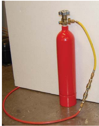
Vacuum suction of the filling hose
