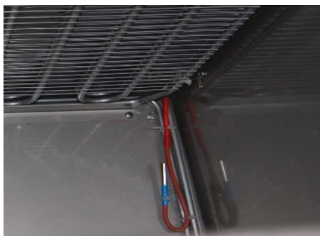
Mounting of the sensor in the freezer
