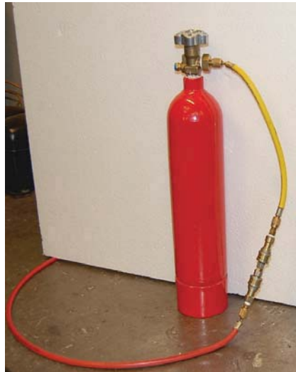
Vacuum suction of the filling hose
