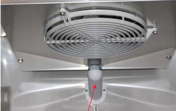
Remove the drain pipe
