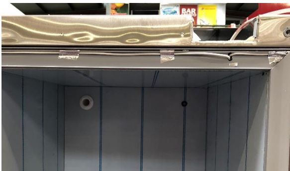
3- Disconnect and remove the heater
