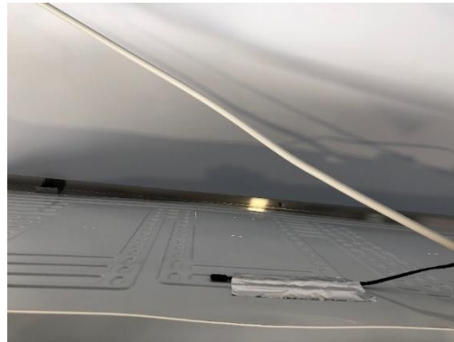
2-Find the probe on the back of evaporator
