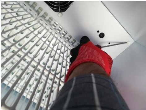
1- Remove plastic cover from screws
