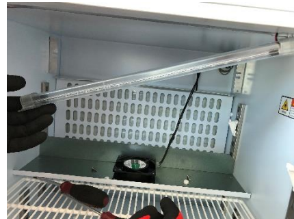
2-Pull out led protection
