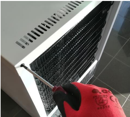
1- Remove screws on back of top panel
