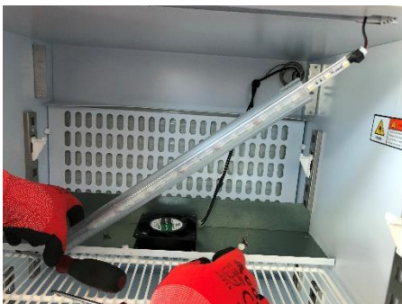
3-Remove led Protection and take led stripe
